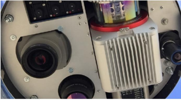
The pod, which holds the LIDAR, Phase One camera and IMU/GNSS system can easily be swapped between different helicopters on a moment's notice. This is especially useful, because Birdview takes on projects outside of Italy and rents aircraft for the purpose. They can pack up their system and attach it to a rented aircraft, perform the project and return to Italy for the processing.
